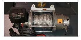
Winch cable should be inspected after every use to ensure no damage had occurred during the previous use.
